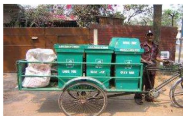
Figure A2-2: Recommended rickshaw van with containers and bags for inorganic waste
