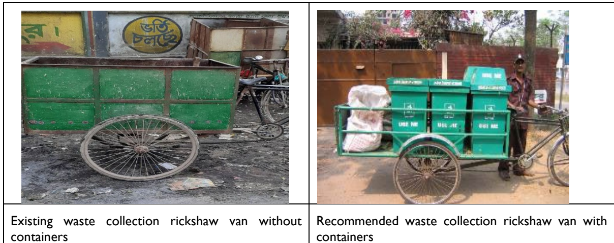
Figure 3.9 Existing waste collection van and recommended van with containers Source: Consultant's Assessment
