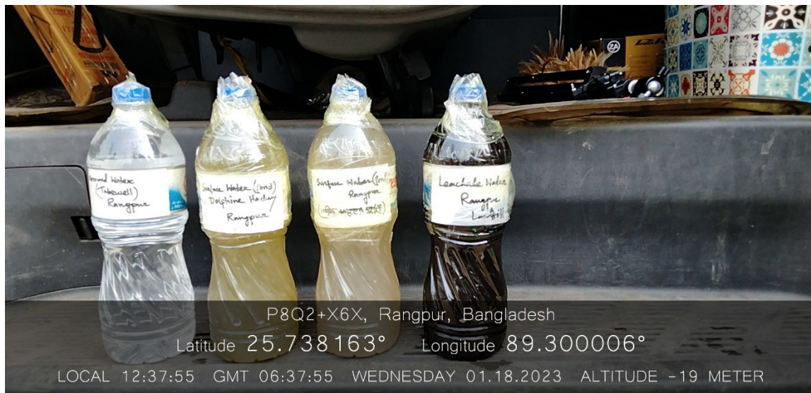
Figure 4.21 Groundwater (L), surface water (M 2 bottles) and leachate water (R)
