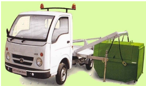
Figure 3.15: Proposed waste collection small truck to carry containers
