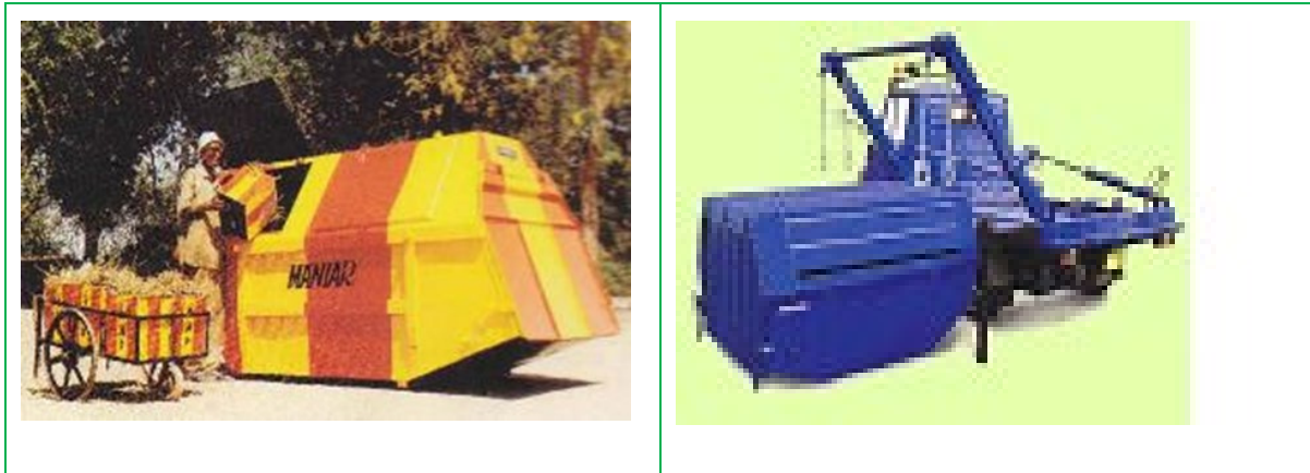
Figure 3-5 Proposed Demountable Containerized Bins
