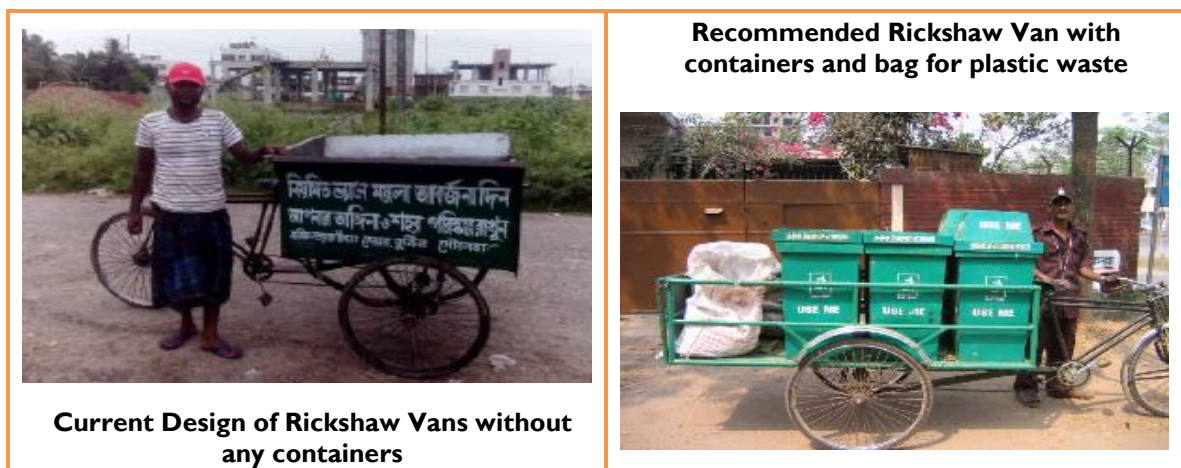
Figure 3-4 Proposed Rickshaw Van For Primary Waste Collection
