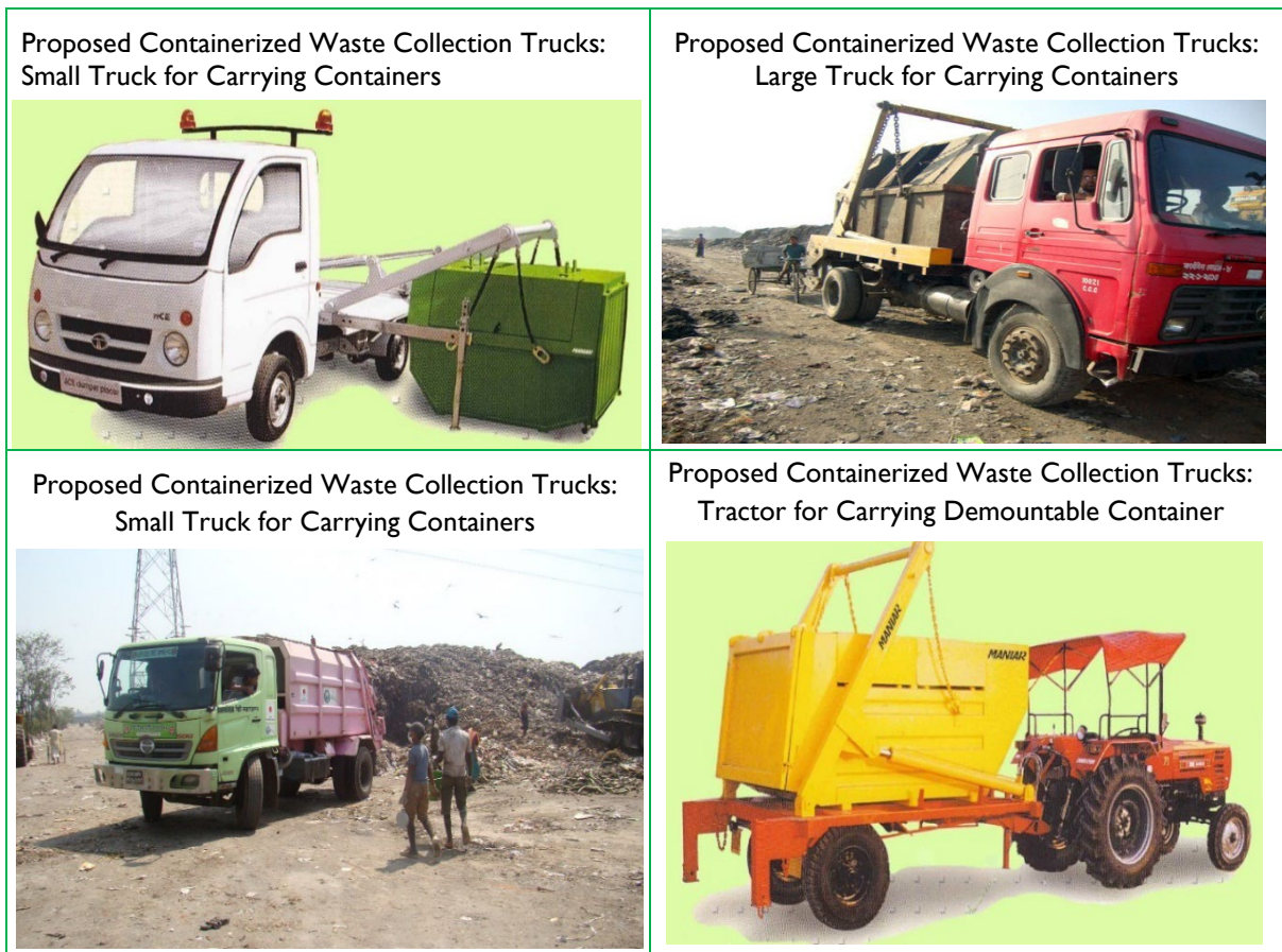
Figure 3-6 Proposed Containerized Waste Collection and Transportation System Source: Consultant's Assessment
