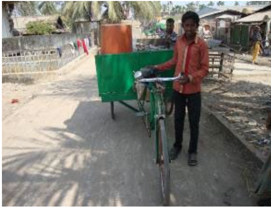
Figure 3-10: Current Design of Rickshaw Vans with container Source: Consultant's Assessment
