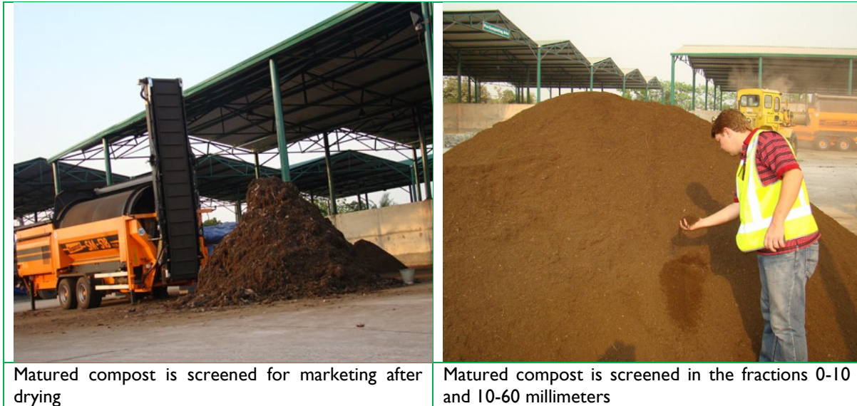
Figure 3-26: Screening of matured compost
