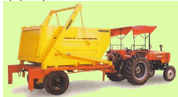
Figure 3-16: Proposed Containerized Waste Collection Trucks: Tractor for Carrying Demountable Container
