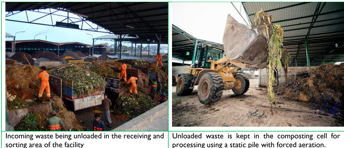
Figure 3-24: Figure showing unloading of waste and transferring them into composting cell
