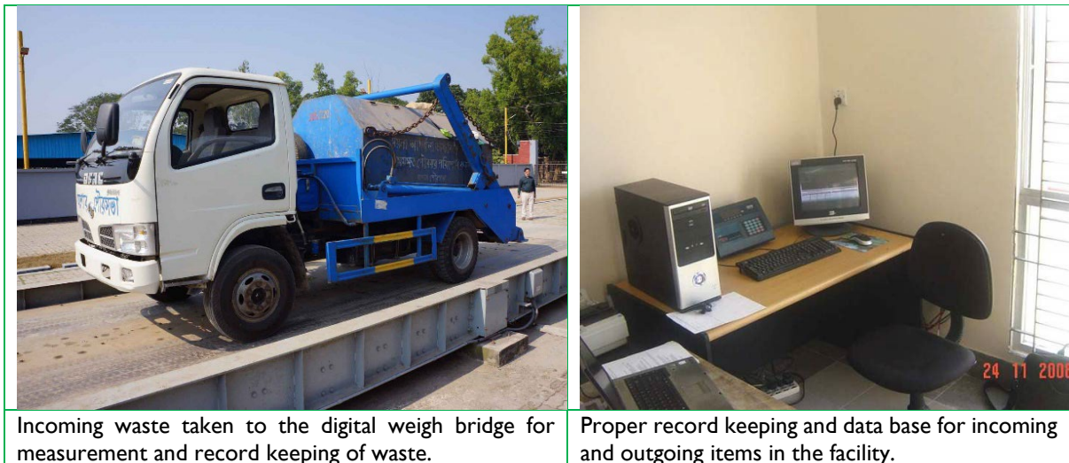
Figure 3-23: Record keeping of incoming waste through digital weigh bridge
