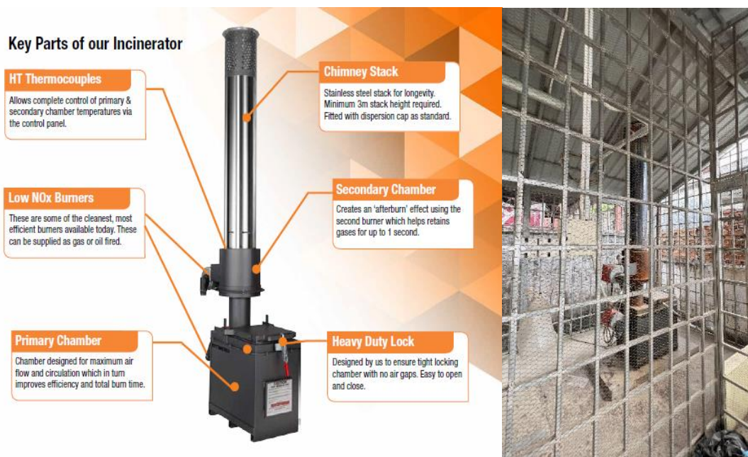
Figure IV-1. Key parts of the incinerator used by NAHPRI lab and photo
