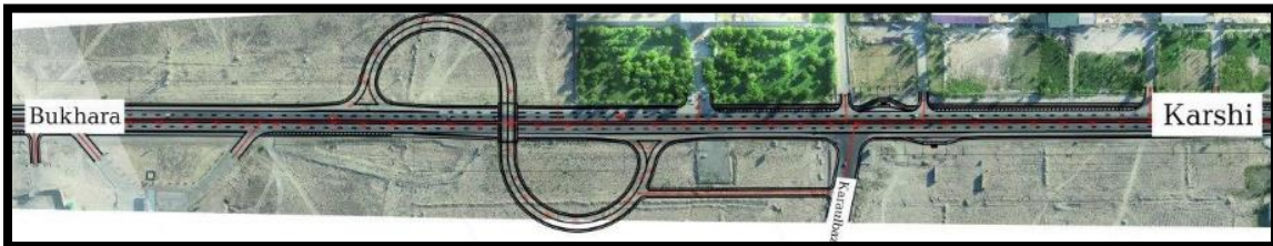
Figure 3.8: New projected interchange on 170 km
