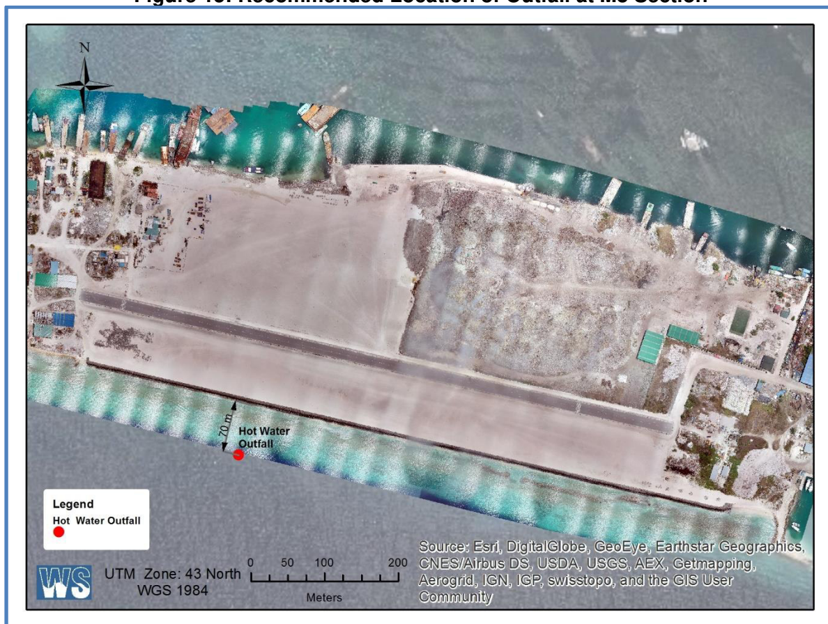
Figure 15: Recommended Location of Outfall at M8 Section
