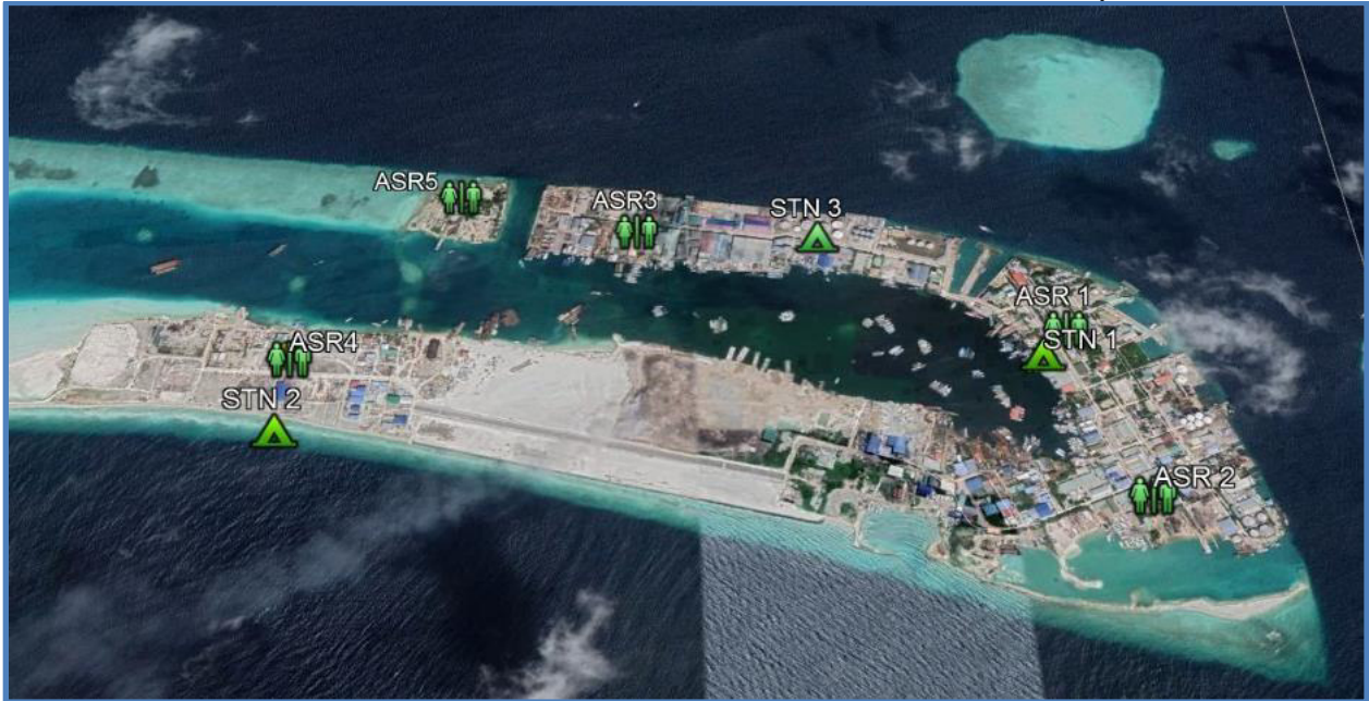
Figure 3: Recommended Ambient Air Quality Monitoring Sites at Thilafushi (AERMOD's confirmation of recommended sites by AUSTAL2000, plus additional recommended sites at ASR2, ASR3 and ASR5 locations)
