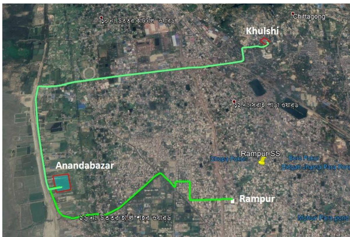
Figure 3.4: khulshi-Anandabazar (New Mooring)-Rampur 230kV double circuit UGTL
