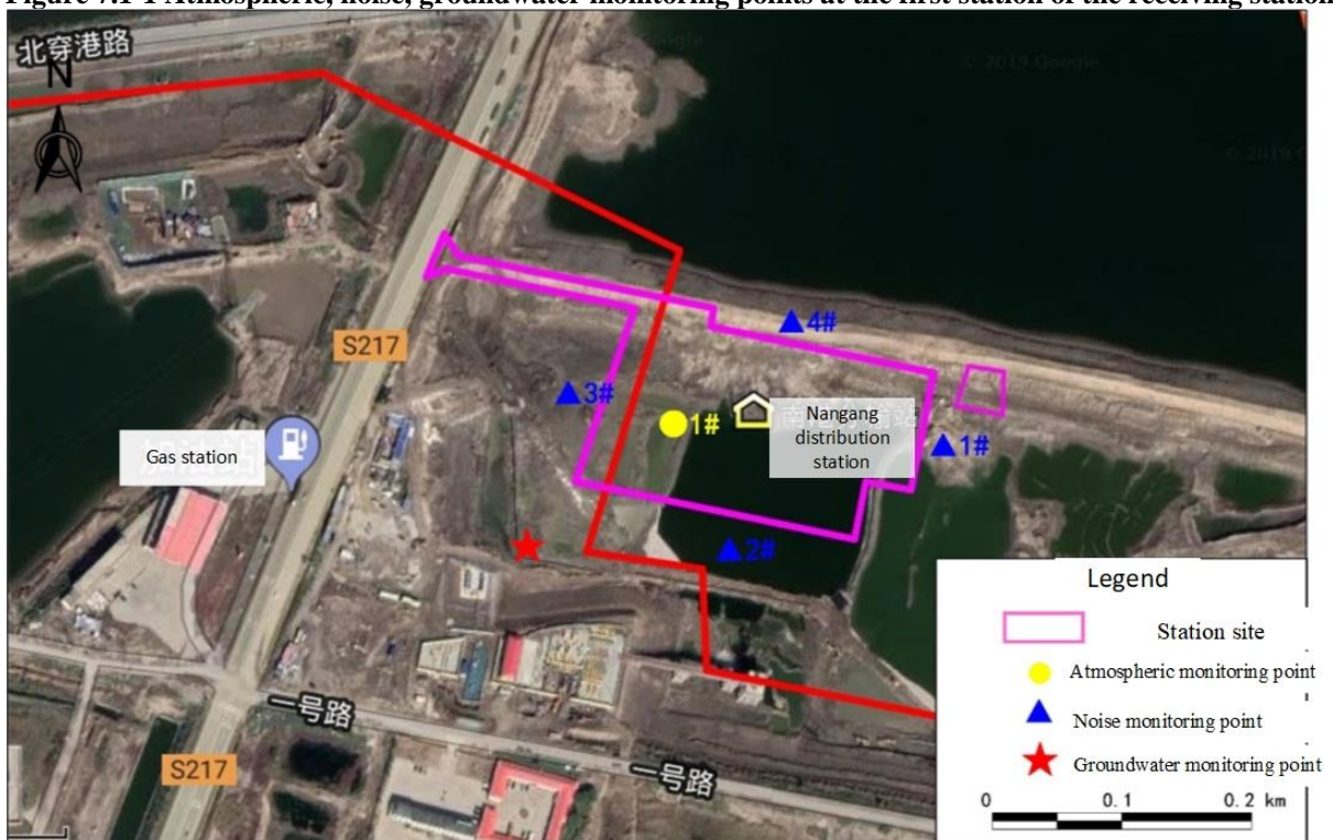
Figure 7.1-2 Atmospheric, noise and groundwater monitoring points at Nangang Substation
